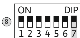
Fig. 16: DIP-brytare 1: intern summer
