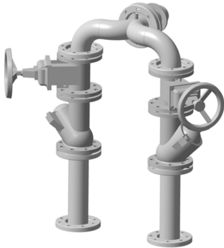
Fig. 6 DC, pipe system with direct, common outlet
