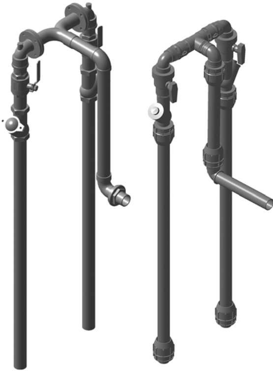
Fig. 10 GC, pipe systems with goose neck, PE D63, stainless steel DN 50, and common outlet
