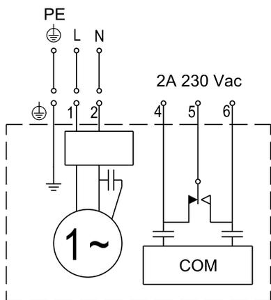
Fig. 29 Wiring diagram for single-phase AUTO<sub>ADAPT</sub> pumps
