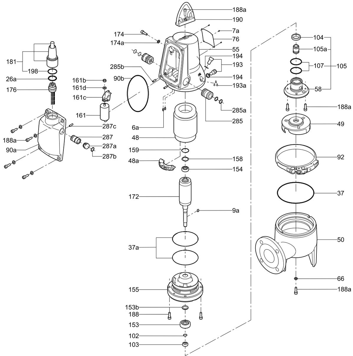
Fig. 24 Exploded view, SLV.65.65.09/11/15 AUTO<sub>ADAPT</sub>
