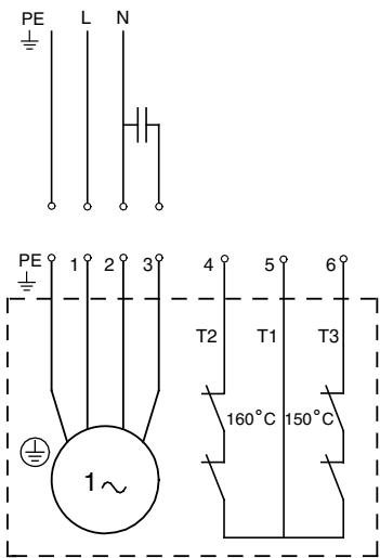
Fig. 28 Wiring diagram for single-phase pumps
