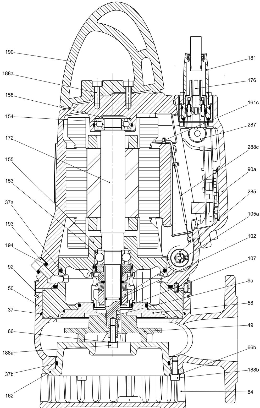
Fig. 13 Sectional drawing, DP10.65.26 AUTO<sub>ADAPT</sub>
