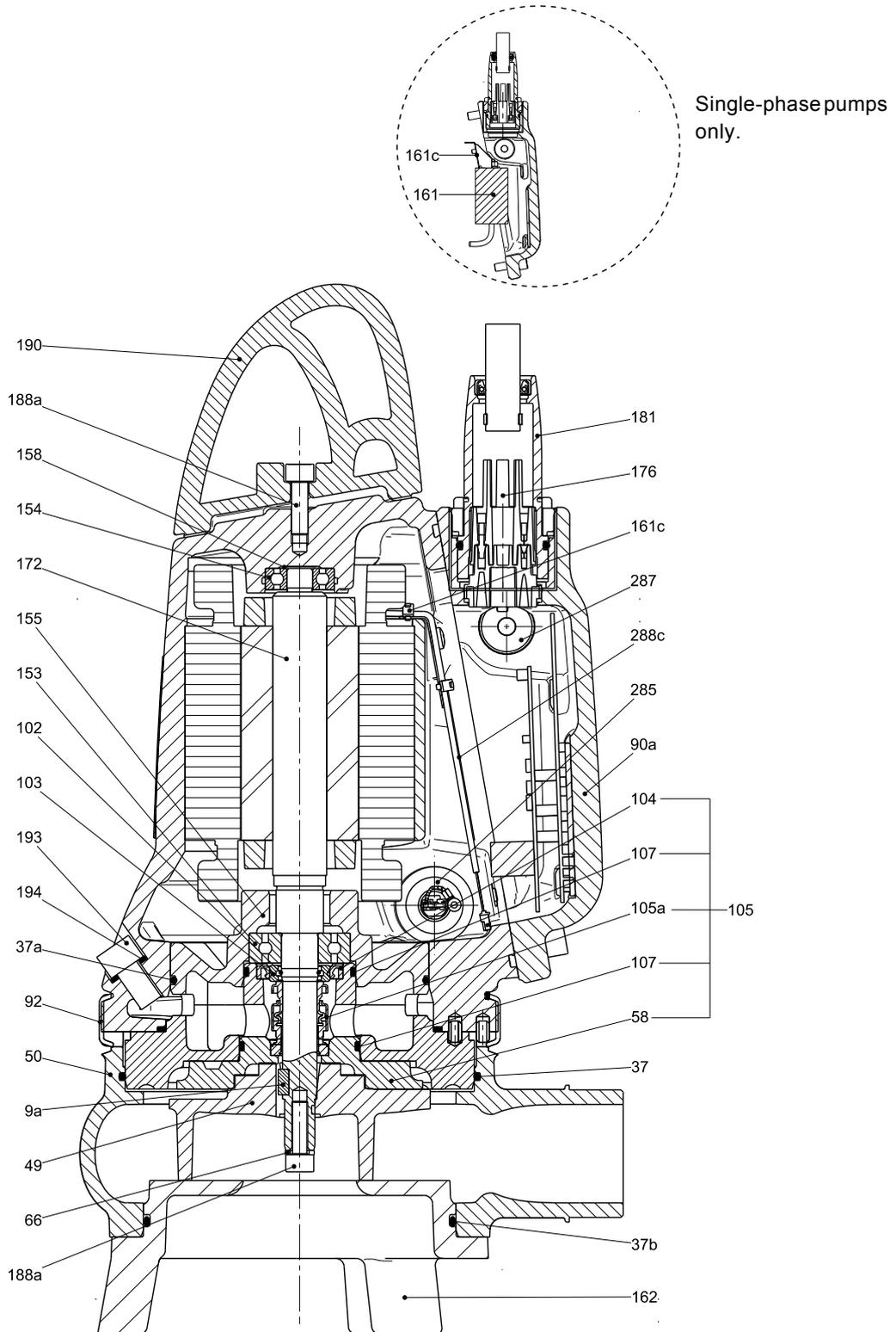
Fig. 15 Sectional drawing, EF AUTO<sub>ADAPT</sub>
