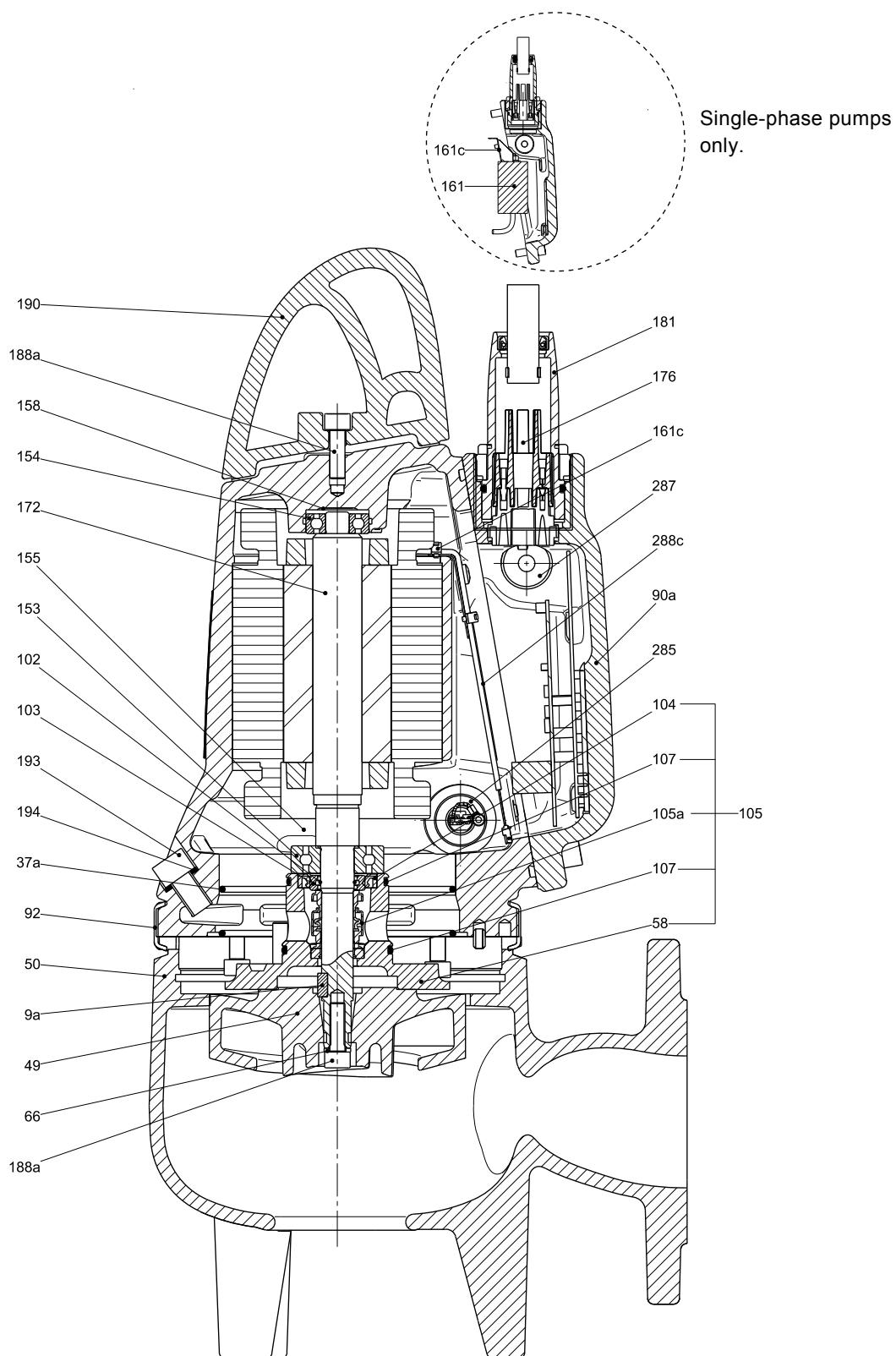
Fig. 23 Sectional drawing, SLV.65.65.09/11/15 AUTO<sub>ADAPT</sub>
