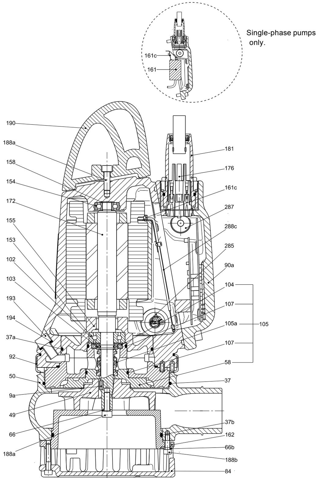
Fig. 11 Sectional drawing, DP10.50.09/15 AUTO<sub>ADAPT</sub>
