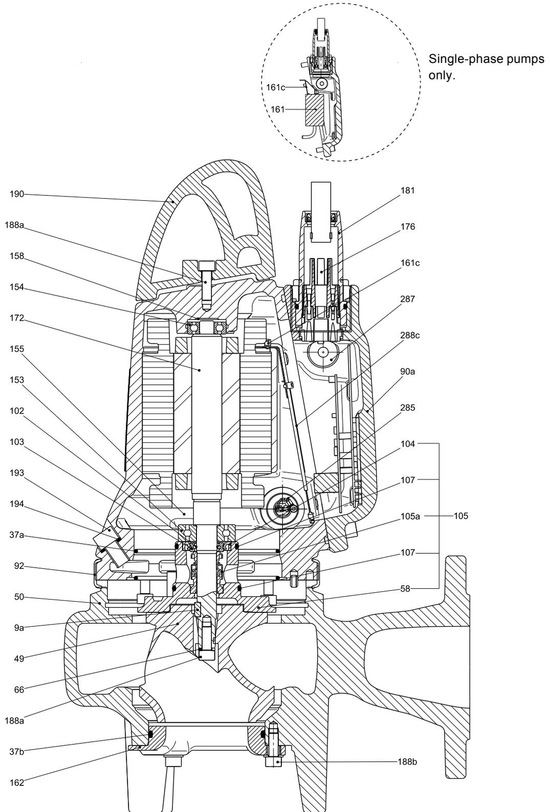
Fig. 21 Sectional drawing, SL1.50.65.09/11/15 AUTO<sub>ADAPT</sub>
