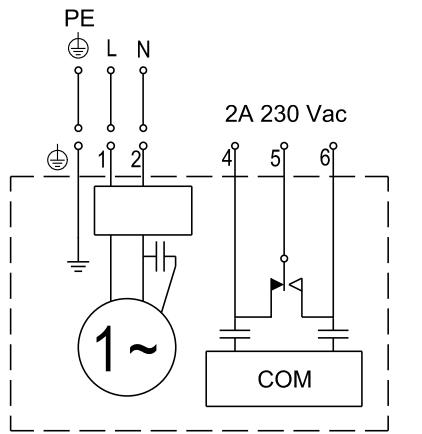
Fig. 29 Wiring diagram for single-phase AUTO<sub>ADAPT</sub> pumps
