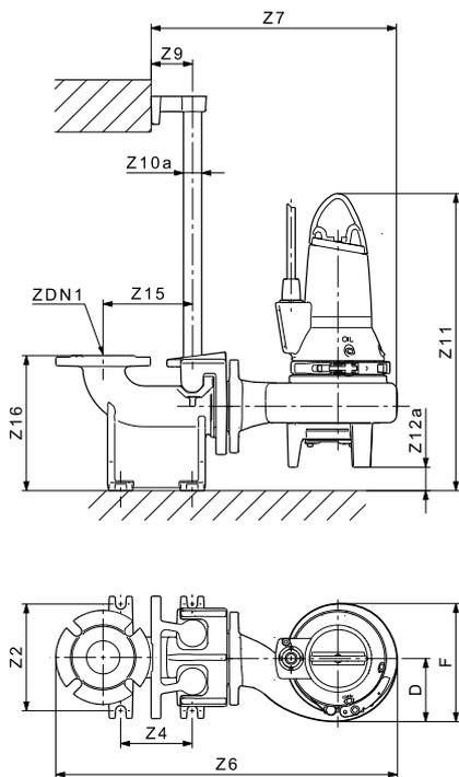
**Fig. 44** One-pump installation on auto-coupling
