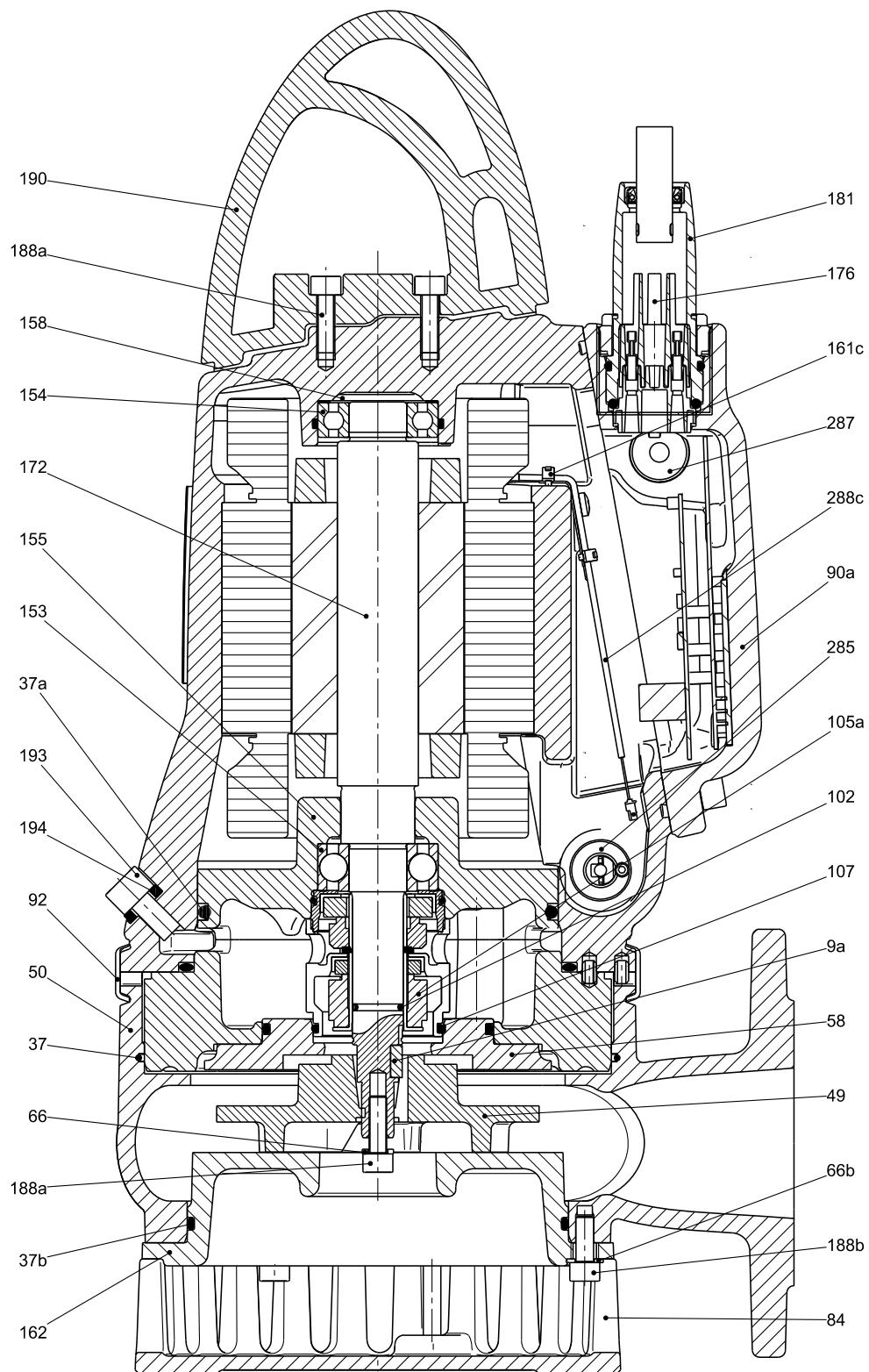
Fig. 13 Sectional drawing, DP10.65.26 AUTO<sub>ADAPT</sub>
