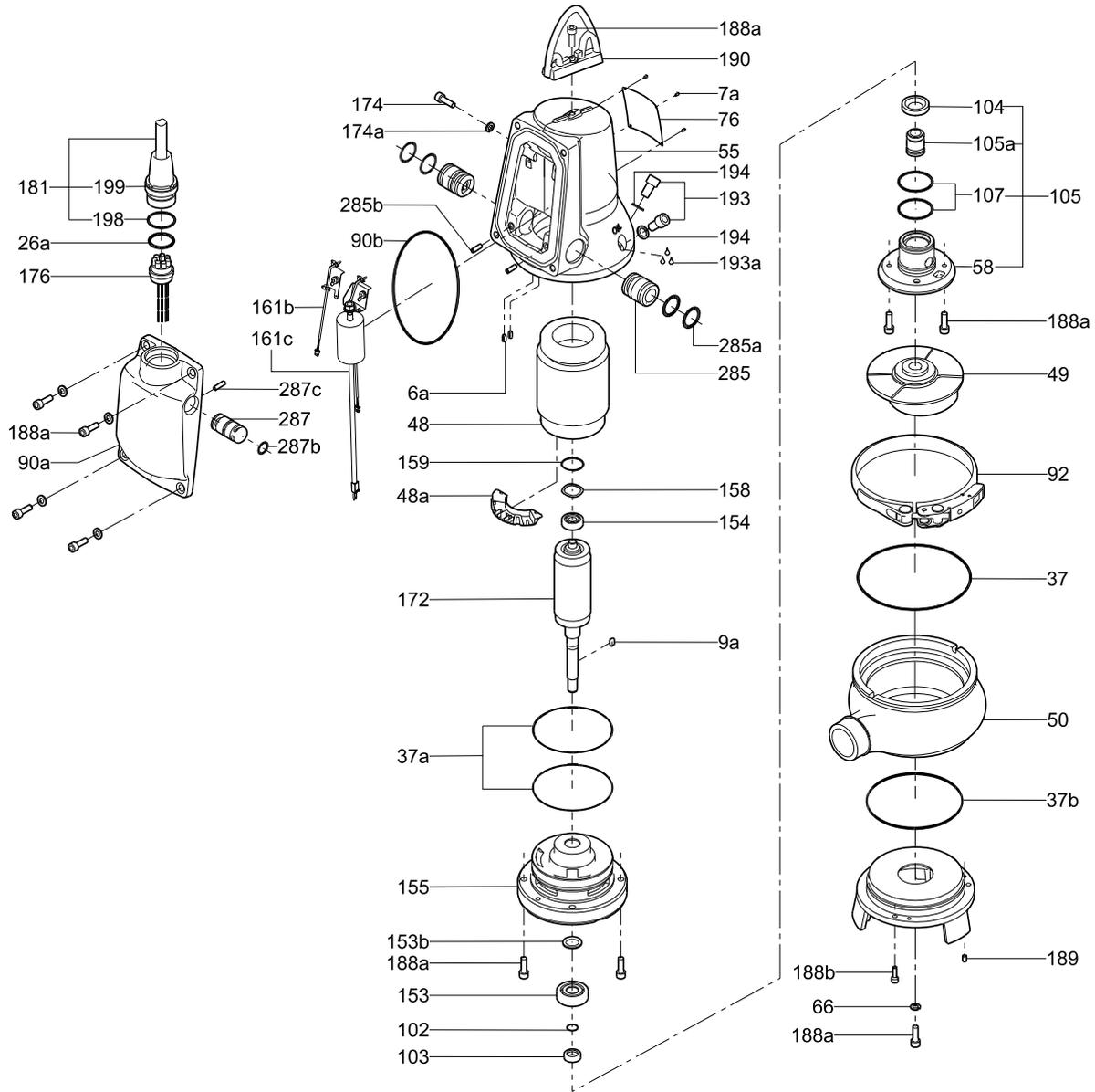
Fig. 16 Exploded view, EF AUTO<sub>ADAPT</sub>
