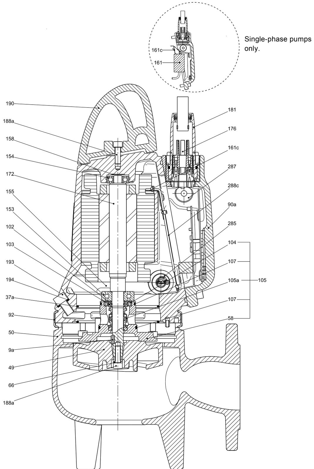
Fig. 23 Sectional drawing, SLV.65.65.09/11/15 AUTO<sub>ADAPT</sub>
