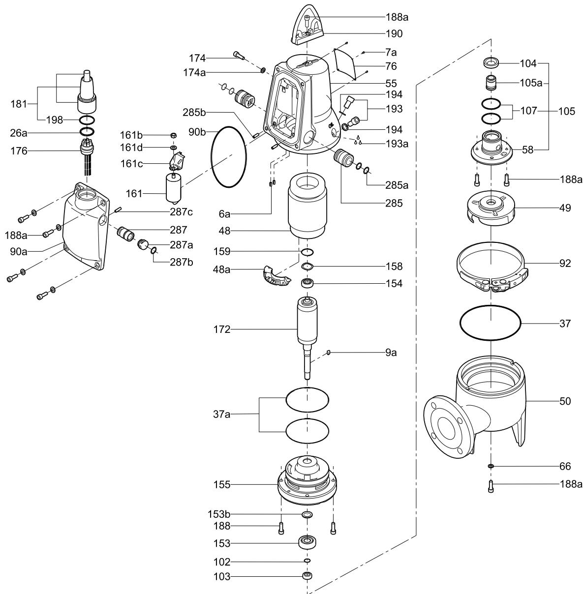
Fig. 24 Exploded view, SLV.65.65.09/11/15 AUTO ADAPT
