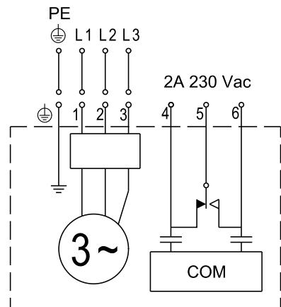
Fig. 31 Wiring diagram for three-phase AUTO<sub>ADAPT</sub> pumps
